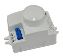
SK603 is a moving object sensor that can detect range of 360° and it's working frequency is 5.8G. The advantage of this product is stable working state (stable working temperature: -15°~+70°C), SK603 adopts a microwave sensor (high-frequency output<0.2mW), so that it is safe and performs batter than infrred sensor.
